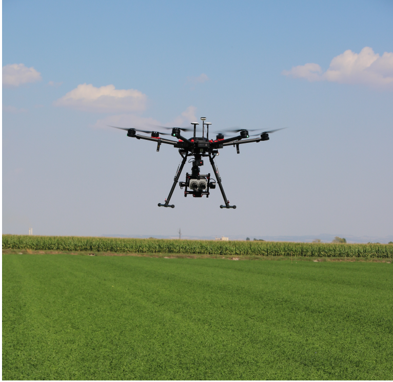
Figure 3.1: SIF dual-camera system mounted on a DJI Ronin MX gimbal
