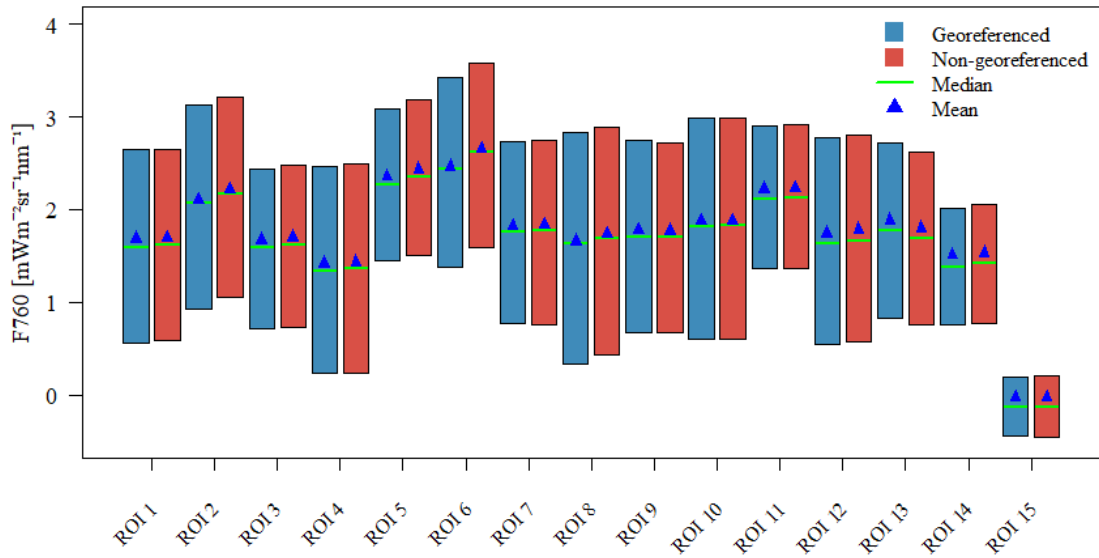
Figure 3.7: Comparison of the distribution of pixel F_{760} values in 15 ROIs (Figure 3.2) between the original raster (non-georeferenced) and the georeferenced raster from mosaic 2a. The dividing green line is the median, and the blue triangle is the mean.
